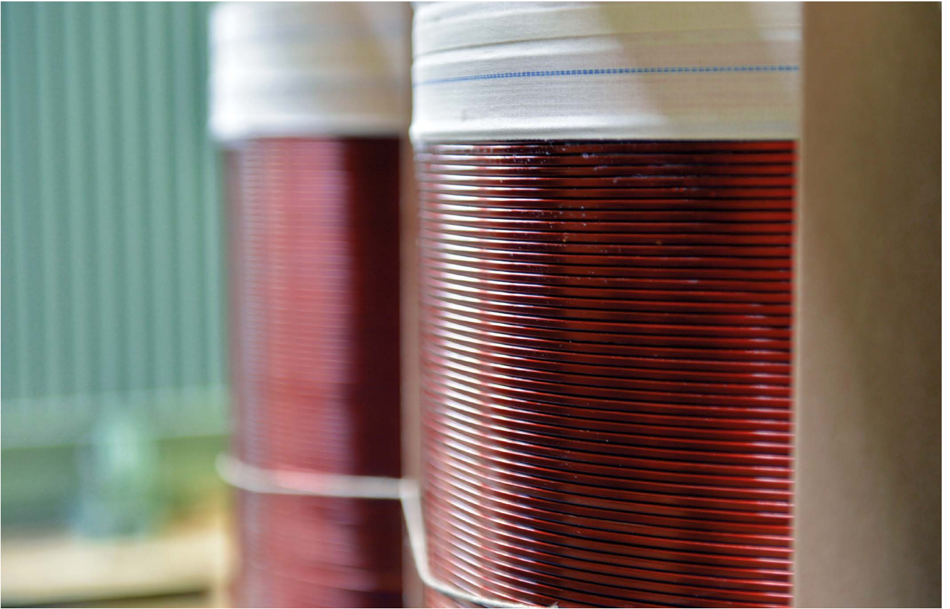
Winding of a distribution transformer
