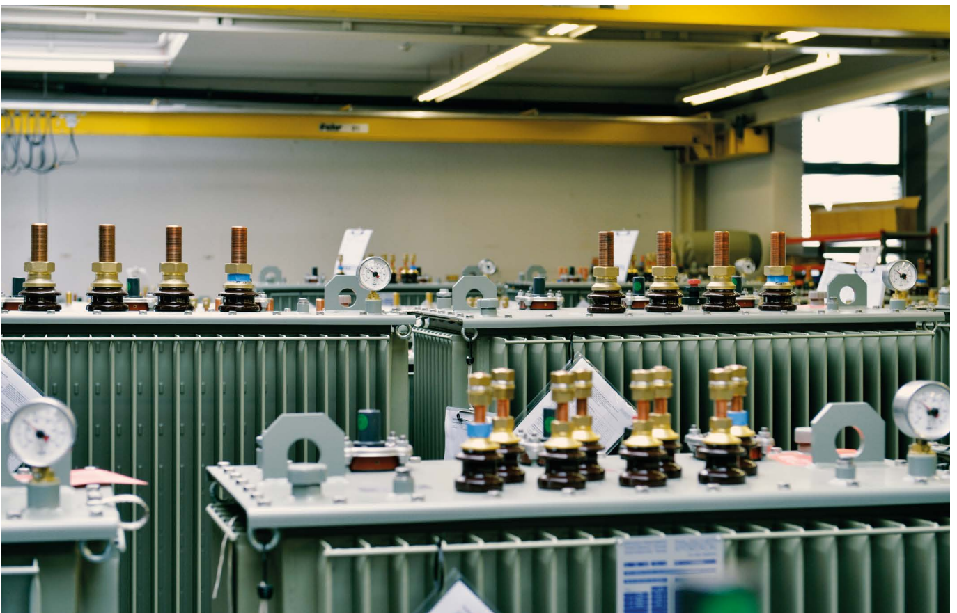
Distribution transformers prior to delivery
