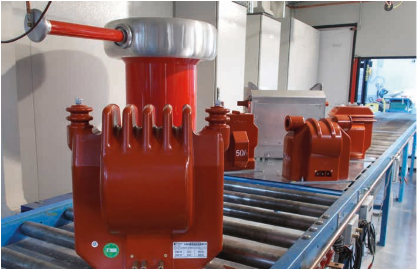
Instrument Transformers at Laboratory
