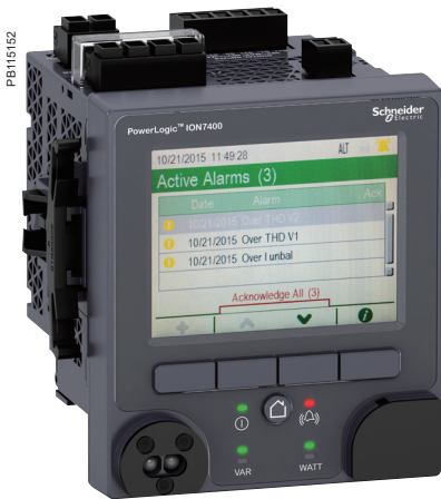
PowerLogic ION7400 meter showing active alarms.
