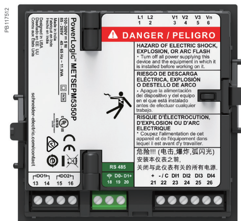
Rear view of PowerLogic PM5350P
