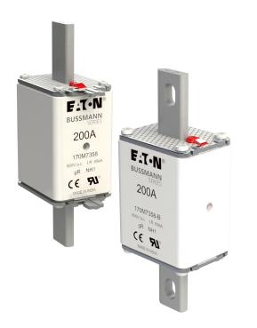
Eaton's Bussmann<sup>™</sup> series 800 Vac NH size fuses are specifically designed to meet the needs of branch circuit and transformer protection in photovoltaic (PV) inverter systems. The fuses are capable of interrupting low overcurrents associated with faulted PV systems (such as reverse current or multi-array faults).
