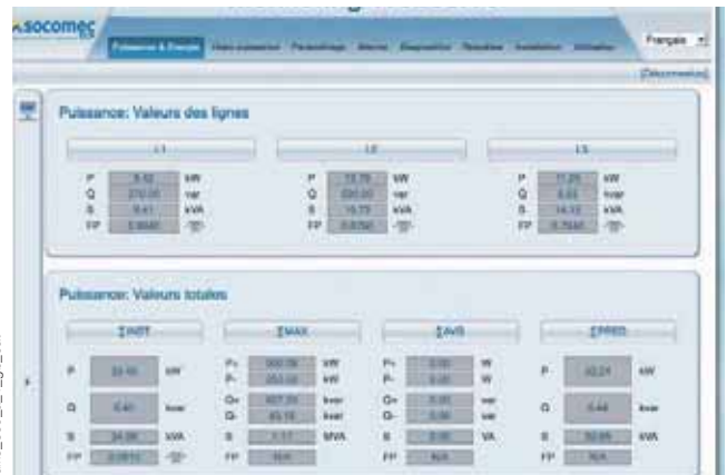
Display for viewing instantaneous and average power measurements and energy consumption.
